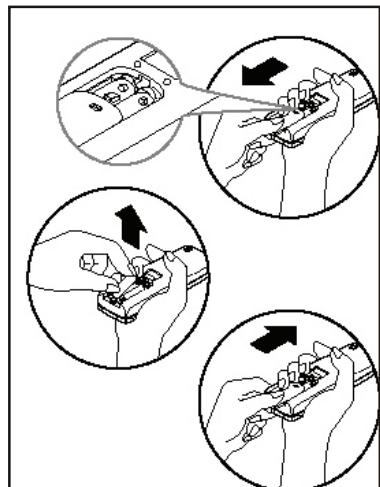
The remote controller is powered by two dry batteries(R03/LR03X2) housed in the rear part and protected by a cover.
