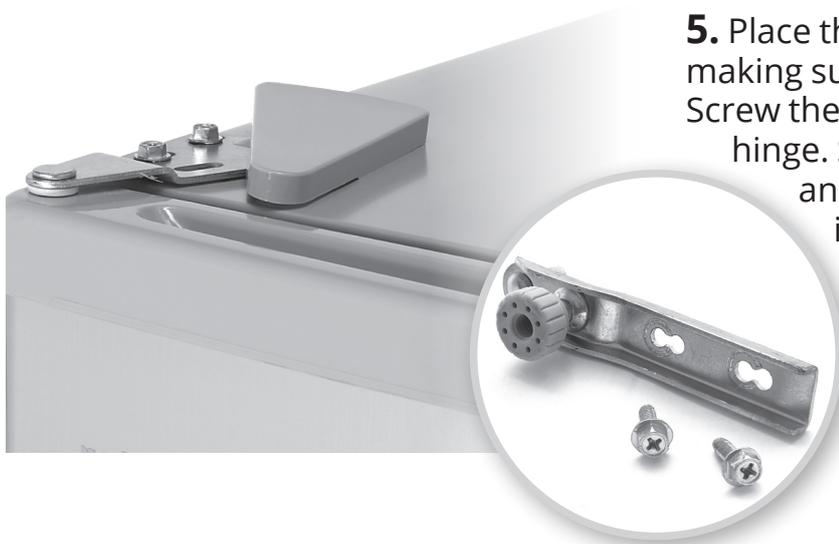
**5.** Place the door on the desired side making sure it is in its upright position. Screw the top two screws of the door hinge. Slightly tilt, for better positioning, and screw the bottom hinge into place, and also screw the removed foot on the other side. Once completed clip on the top plastic cap.
